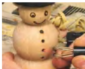
▲ Pic.13 Create the eyes, mouth and buttons using a pyrography machine, or you could turn them if you wish
